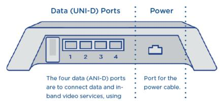
The <u>nbn</u> connection box is wall-mounted and has four Ethernet ports that can deliver internet data. It requires power to operate and can only be installed by an <u>nbn</u> approved technician.
