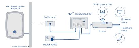
End users can connect their devices directly to the <u>nbn</u> connection box via an Ethernet cable. if they prefer to connect via Wi-Fi, they'll need to connect their own router, or one supplied by their Retail Service Provider, to the **nbn** connection box.
